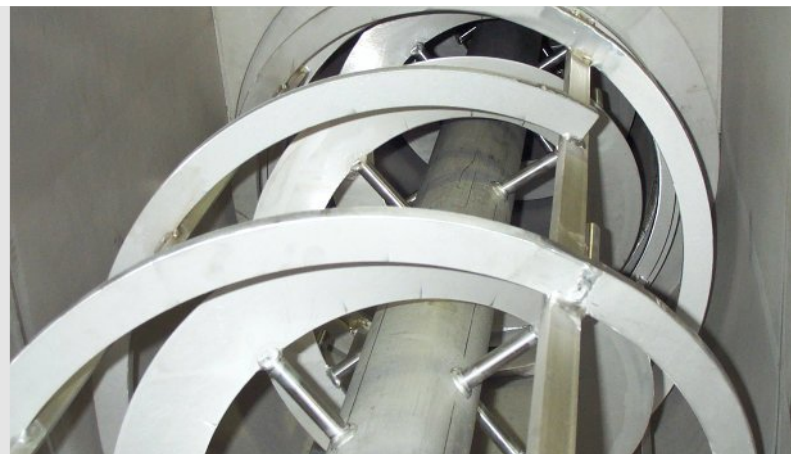
Shafts of a continuous flow mixer
