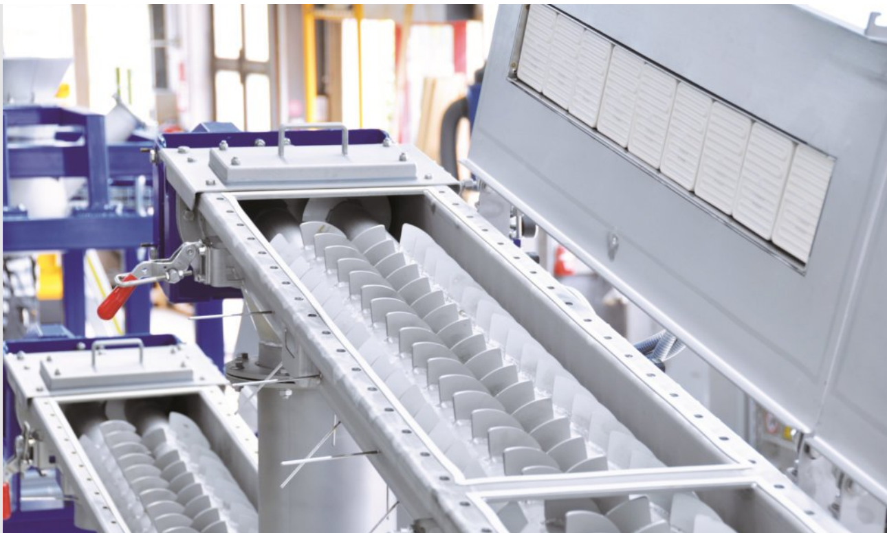
Double shaft mixer with radiant heaters in the cover
