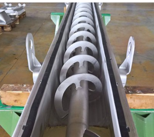
Screw conveyor with ribbon flights
