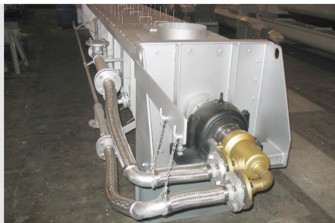
Rotary joint at the end bearing
