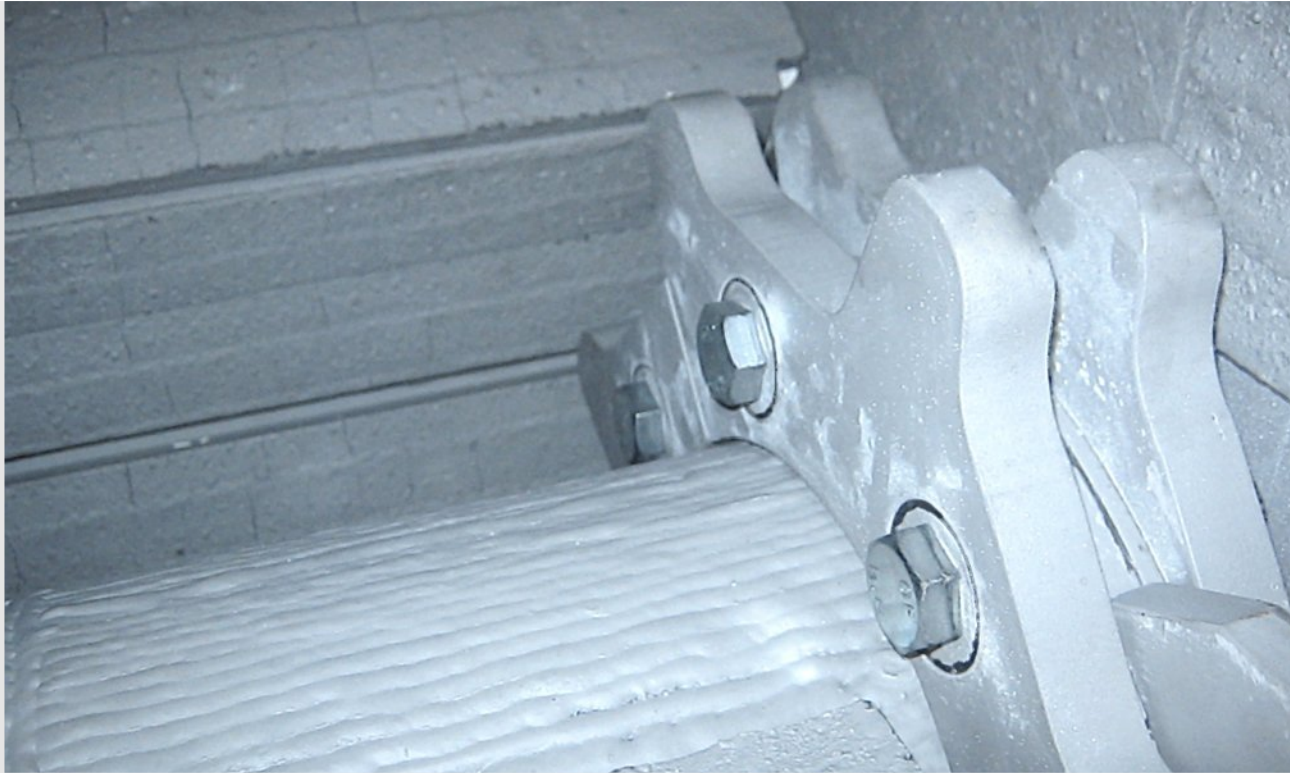
Material loop and shaft with wear protection
